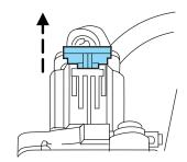
2. Loosen the hose clamp located closest to the air cleaner.
